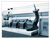
**100% Leak Tested** Every cylinder-head cover is tested for sealing integrity.
