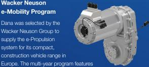
a comprehensive electrodynamic system from Dana, encompassing the Spicer Electrified™ eSG101 e-Transmission, Dana TM4™ SRI 200 motors, AC-X1 inverters, an APC 300 series controller, and accompanying software for managing vehicle traction and operations.
