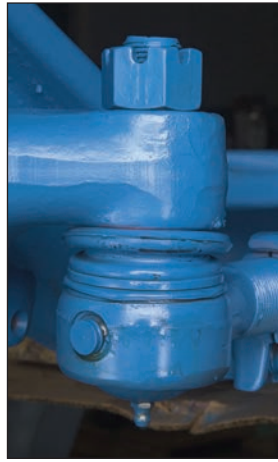
Patented purge valve tie rod rod end with sealed boot.
