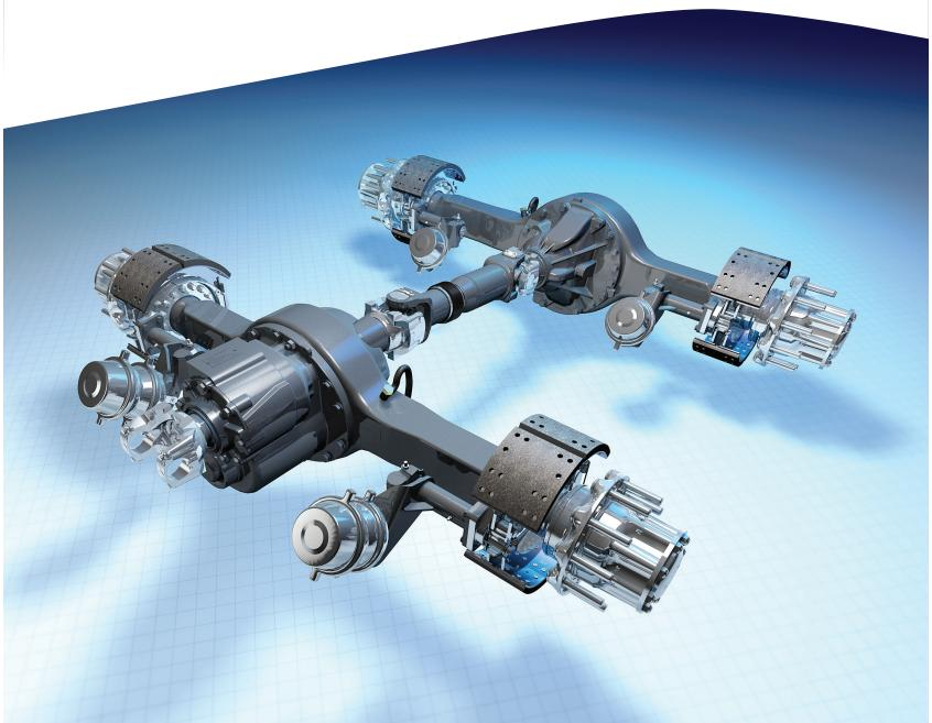
**The Spicer® AdvanTEK® 40 tandem axle** – the most durable and reliable axle for Class 8 applications, featuring highly efficient, robust AdvanTEK® gearing. This innovative product has significant competitive advantages that allow it to withstand 30 percent higher input torque and enable more than 2 percent improved vehicle efficiency.
