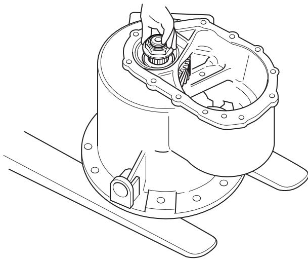
11. Align a 6" x 6" x 6" wood block under the drive pinion, then lower the carrier and pinion assembly into a press so that it is supported by the block.
