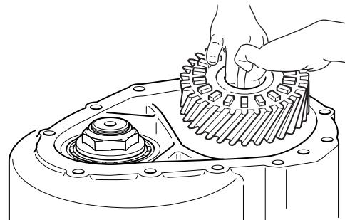
6. Install helical side gear thrust washer.
