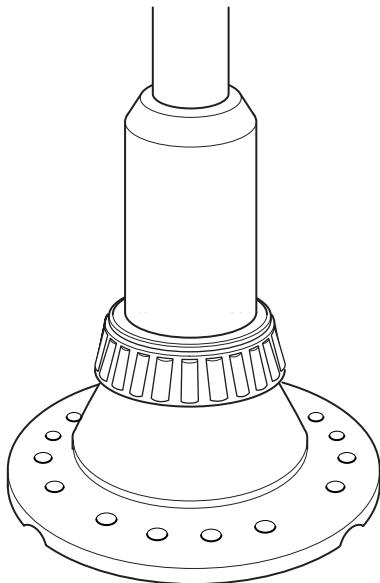
2. Place the plain half side of the differential case on a malleable surface.
