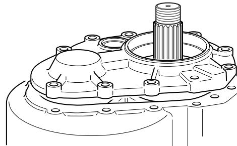
15. Install input shaft bearing adjuster, adjust inward until snug against the bearing cone.
