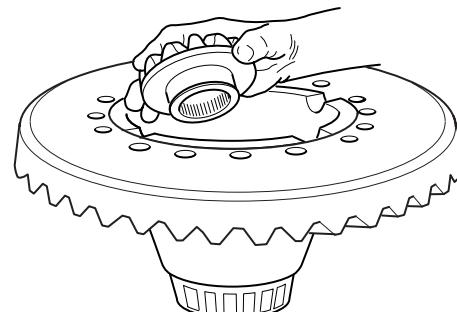
4. Place a block under the plain half, use a rubber mallet to remove the ring gear.
