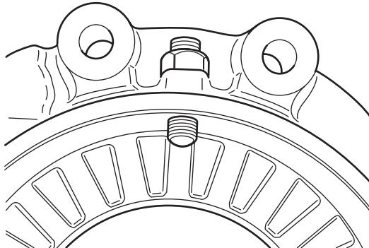
14. Input cage is threaded into the PDU cover, use the proper tool to remove the cage from the cover.
