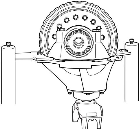
8. Use Dana's wheel diff. bearing adjustment tool (part number 513061) to back off the threaded cups and remove.
