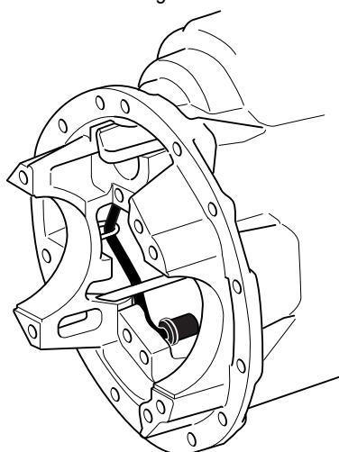
4. Fully press the manifold assembly into position.
