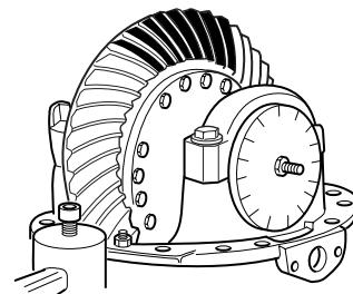
17. With the carrier mounted in a head stand, roll the carrier on its side.
