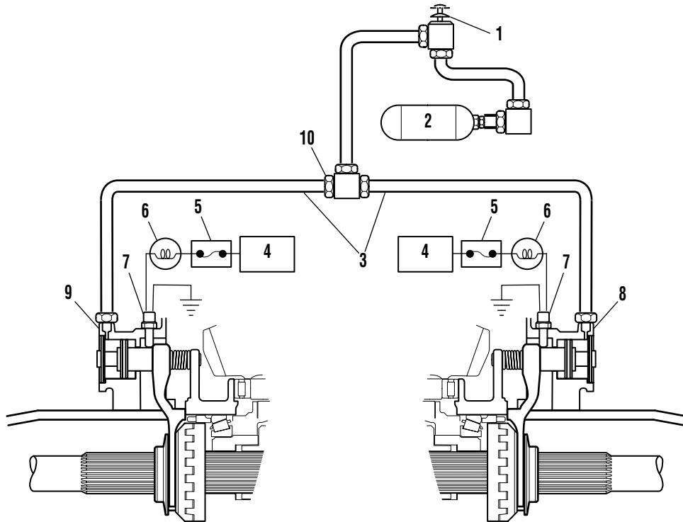
1 - Cab-mounted control valve (plunger in—valve open)
