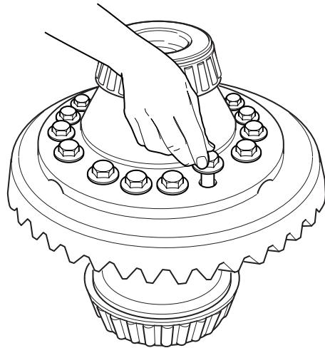
8. Install the flange half of the case. Align the capscrew holes.
