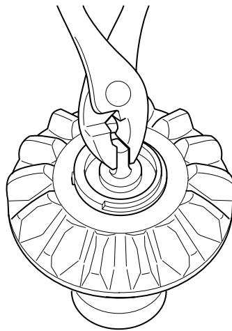
4. Remove the output side gear bearing cup from the carrier with the proper bearing puller tool.
