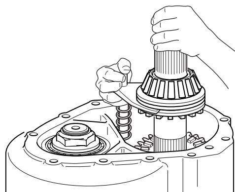
10. Remove the thrust washer and helical side gear.
