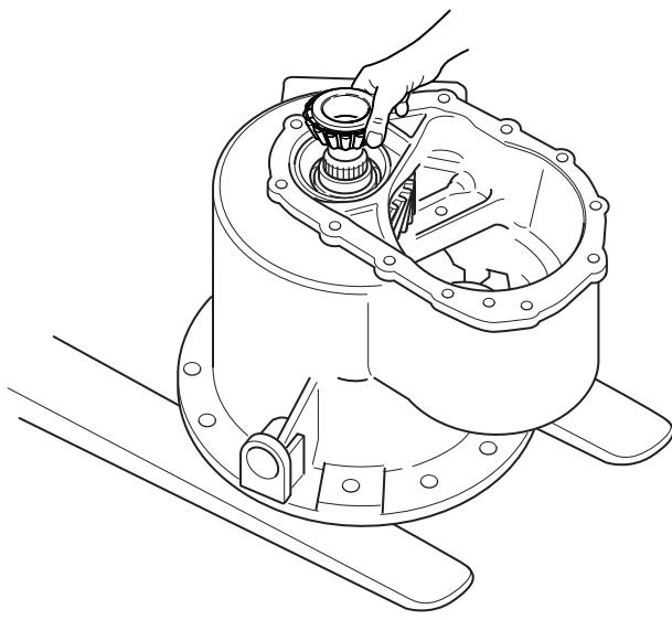
10. Install a pinion nut finger tight. This will hold the pinion in place while it is positioned into the press.
