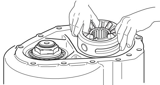
5. Install the helical side gear so that the clutch teeth are facing upward in the carrier.
