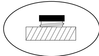
4. Insert hose onto fitting, long end down.
