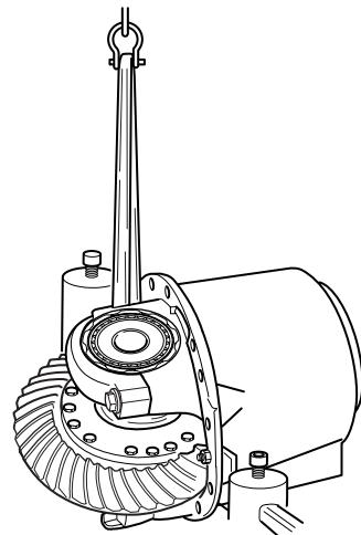
20. Use the correct socket and a breaker bar to rotate the differential. The differential should be hard to turn. Rotate the pinion until the ring gear rotates 3 or 4 times in both directions. See page 45 for descriptions of correct pattern position for new and used gearing.
