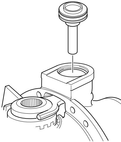
4. Remove the shift fork and sliding clutch assembly.
