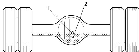
1 - With axle on level surface, fill housing with oil to bottom of plug
