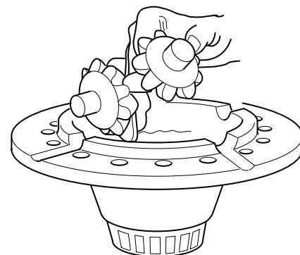
5. Install the flange half side gear. Apply a thin coat of oil to the mating surfaces.
