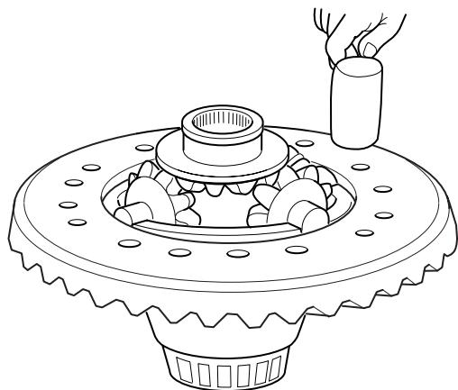
9. Install the ring gear capscrews.
