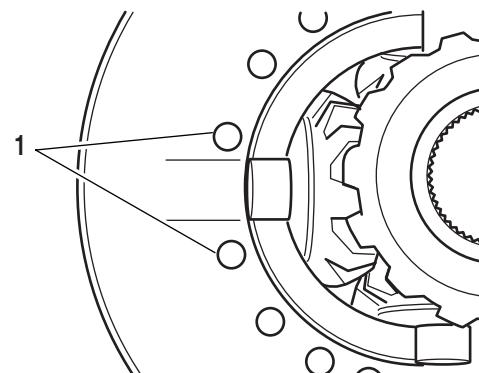
1 - Match spacing of holes on each side of spider slots
