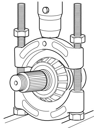
b. Mount the puller horizontally to press the bearing from the pinion.
