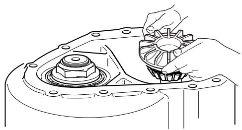
13. To replace the input bearing cup, back off the bearing cage locking fastener or jam nut and stud.
