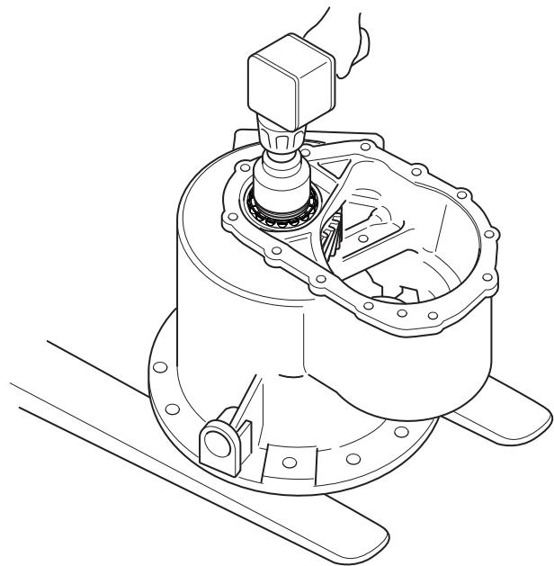
17. Secure the carrier in a head stand, rotate carrier so the pinion nut can be torqued.
