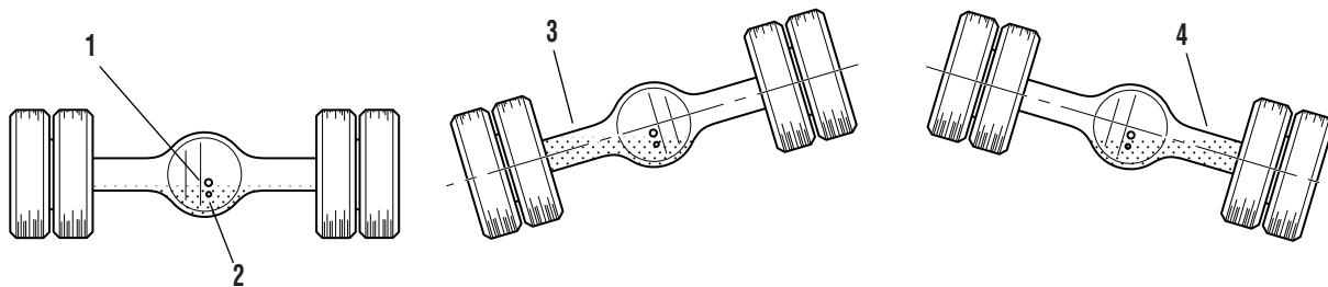
1 - With axle on level surface, fill housing with oil to bottom of plug
