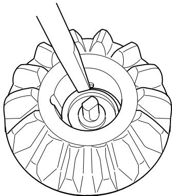
3. Remove pump from the output side gear.
