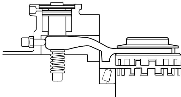
4. Lubricate piston and o-ring with silicone grease. Install shift piston assembly into cylinder. Position piston with small diameter hub toward closed end of cylinder.
