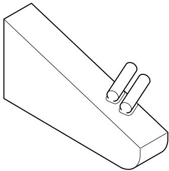
18. Install the wedge between the carrier wall and the teeth of the helical gear.
