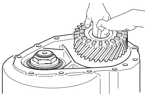
11. Remove the inter-axle differential assembly.
