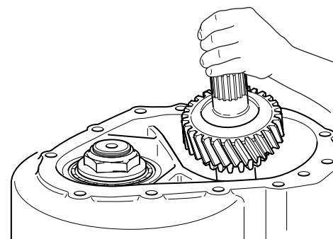
12. Assemble the sliding clutch, shift fork and fork spring to the input shaft and install assembly into carrier. Make sure that the shift fork rod is piloted in the carrier bore.
