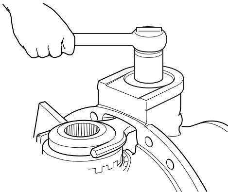
3. Remove the piston push rod from the shift fork.
