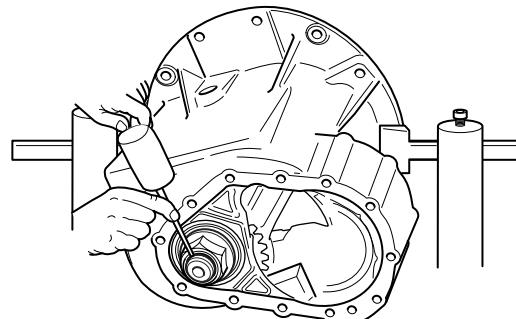
**Note:** Always use a new nut and coat threads with Loctite 277 if not pre-coated.
