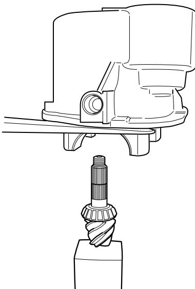
7. To align the splines of the helical gear to the pinion, use a old pinion nut with a metal ring welded to the top, thread onto the pinion. Then lift the pinion while aligning the two splined surfaces.
