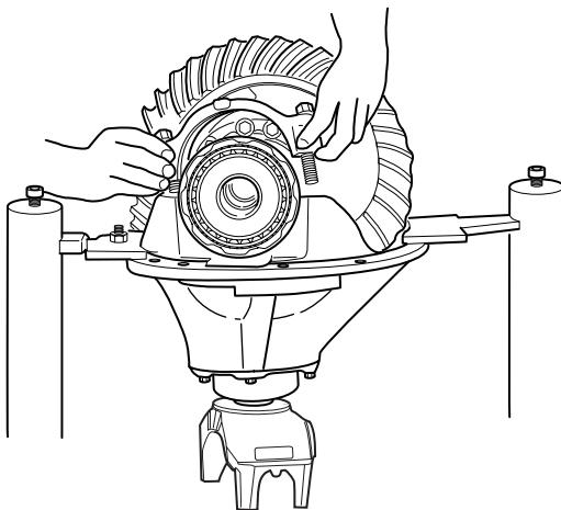
9. Use a chain hoist and the proper strap, lift the ring gear and wheel differential assembly from the carrier.
