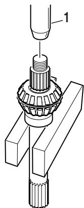
9. Remove output shaft inner bearing cup.
