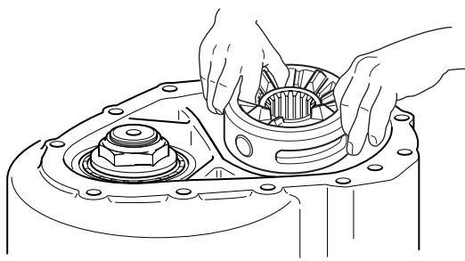
12. Remove the output side gear and pump assembly.
