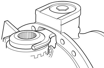
2. Remove the threaded cylinder cap.
