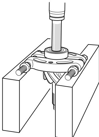
2. Remove the inner pinion bearing cone from the pinion using a split-type puller. Use two procedure steps to remove each bearing.
