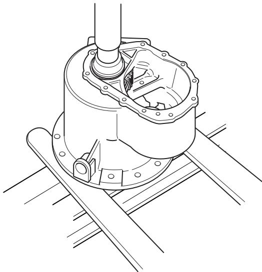
14. With 5 tons of force on the press, you should be able to feel a small amount of drag from the bearing as you rotate the carrier. If the carrier turns with no drag at all, the pinion spacer thickness should be decreased by using a thinner spacer. If the carrier is hard to turn, the spacer thickness must be increased.
