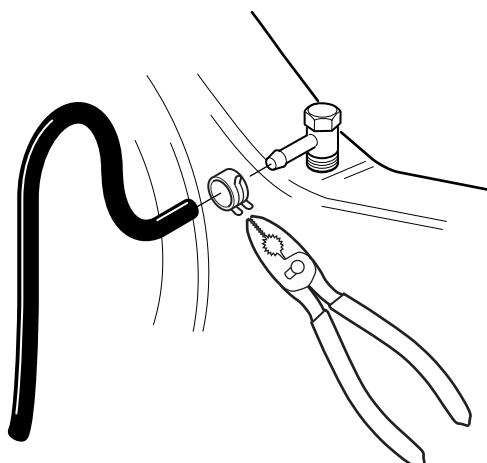
5. Push hose firmly against fitting. Rotate hose to point down.
