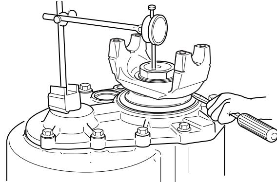
22. Use a punch with a round tip to stake the pinion nuts flange into the machined slot in the pinion shaft. See diagram below.
