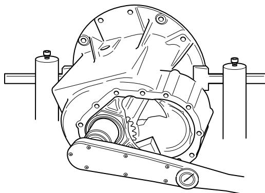
**TIP:** If you are unable to torque the yoke nut correctly, try torquing the nut with the truck wheels on the ground and with the axle shafts installed.
