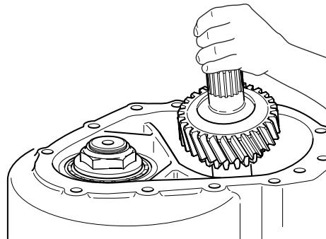
9. Remove the input shaft, sliding clutch, shift fork and spring as an assembly.
