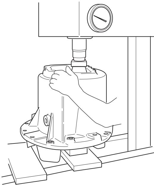
15. Remove the carrier from the press and reinstall the pinion nut.
