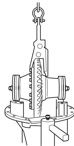
**Note:** There are two ways to make sure that the threaded cups are seated properly. If there is a misalignment, reinstall the differential assembly at a slightly different angle.
