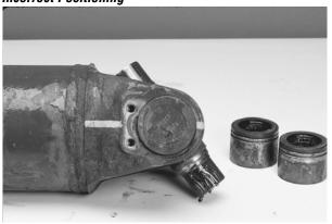
Using an arbor press, press down on the upper bearing cup assembly until the shoulder of the journal cross makes contact with the inside of the yoke ear.
