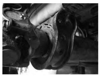
**Note:** If looseness is evident, retighten center bearing bracket bolts. Consult the vehicle manufacturers' specifications for proper bolt torque. Check the alignment of the bracket before tightening the bolts. Bracket should not be skewed.
