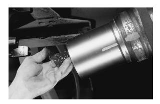
Measure and place a mark 2.25 inches (55-60mm) from yoke shaft shoulder with a marking stick, paint marker or other legible marking device.
