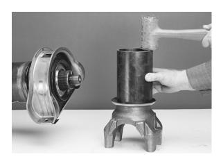
Using a soft-faced hammer, drive the yoke onto midship tube shaft, making sure phasing marks from driveshaft removal procedure are in line. Continue to tap the yoke until it is completely seated against the center bearing.
