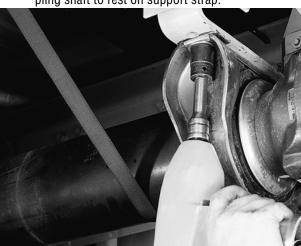
4. Using a puller, follow the tool manufacturer's instructions to remove the yoke and center bearing companion flange. Both the yoke and companion flange are press fit and should **NOT** be removed with a hammer. If either the yoke or companion flange are loose enough to be removed by hand, the entire coupling shaft must be replaced. Remove and discard slinger from the yoke.
