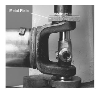
Place a push rod that is smaller than the diameter of the bearing cup assembly under the bearing cup assembly and continue pressing into the yoke cross hole until far enough to install a snap ring.
