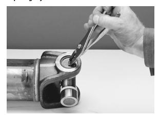
For Quick Disconnect™ Style: Remove spring tab bolts and discard, and remove outboard bearing cap assemblies.
