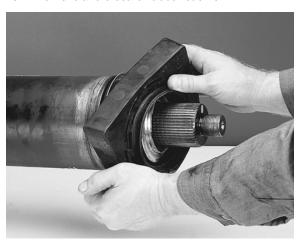
4. Using a puller, follow the tool manufacturer's instructions to remove the bearing assembly from the midship. Discard the center bearing.
