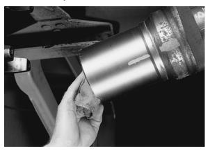
After all traces of grease and cutting solvent have been removed from the yoke shaft and spline sleeve, apply half of the grease provided to the yoke shaft splines and the other half to the spline sleeve, cover the entire splined surface.
