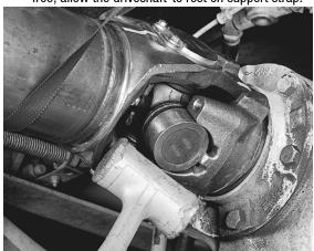
8. Apply a c-clamp around the outboard bearings. Apply grease gun pressure. Completely purge both inboard bearings.
