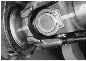
Align the bearing cups with the yoke ears making sure that the cups are evenly spaced between the nibs of the yoke. A soft faced hammer can be used to fully seat the bearing cups into the yoke.
