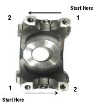
6. Torque strap bolts to specification according to the chart below.
