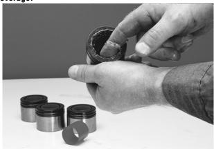
**Caution** - Spicer **DOES NOT** recommend wiping the outside of bearing cup assemblies or yoke cross holes with grease, oil or silicone-based sprays. This could result in bearing cup assembly rotation in yokes.
