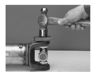
11. Rotate the journal cross to make sure it moves smoothly and freely in the bearings. If not, disassemble and inspect the journal and bearing assemblies for skewed or dropped needle rollers. Reference removal procedrues for universal joints, snap-ring style.
