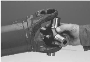
**Note:** Always inspect bearing cups for rollers that may have fallen (downed rollers) out of place before installation.
