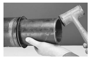
**Note:** If the application requires the installation of a slinger, avoid damage during installation.
