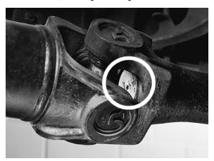
If any of these situations are evident, replacement of the slip yoke and professional rebalancing of the driveshaft is necessary.
