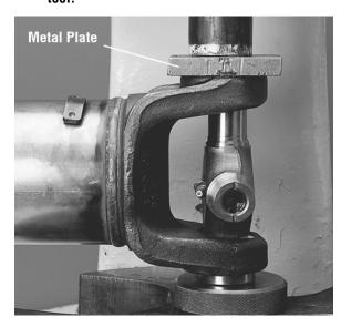
5. Flip yoke 180 degrees. Position the remaining installation heigh tool on the end of another bearing cup assembly. Place bearing cup assembly over trunnion diameter and align it to the yoke cross hole. Push the bearing cup assembly until both installation height tools are flush with the cross hole face.
