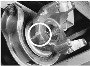
2. Remove midship nut. Discard nut. If washer is damaged, discard and replace. Otherwise, reuse washer.
