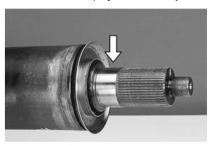
6. If no damage is apparent, remove slinger and discard. Proceed to installation of center bearing.
