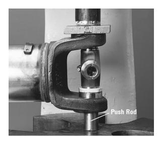
6. Remove yoke from arbor press. Install a snap ring using snap ring pliers.
