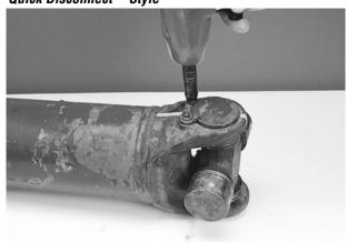
Make sure universal joints cross assembly is not tilted in the yoke. Place bearing cup spacer onto the base of the arbor press and under the yoke. If the arbor is larger than the bearing cup diameter, a smaller diameter push rod will be needed to avoid damaging the yoke or bearing.
