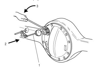
**Note:** The output yoke can be installed when taking end-play measurements.
