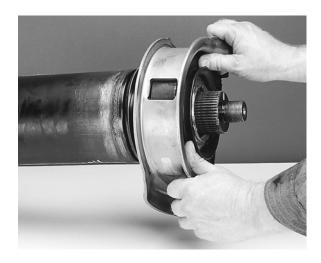
4. Press remaining slinger on end yoke using a section of tubing to avoid damaging slinger.
