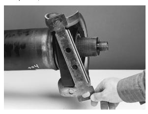
2. Remove and discard the center bearing bracket.
