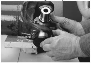
4. Align the yoke in an arbor press with the bearing assembly resting on the base of the press. Cover the yoke ear with a metal plate that has 0.25 inch (6.4 mm) minimum thickness. Push the yoke onto the bearing cup assembly until it is flush with the cross hole face. Do not remove the installation height tool.
