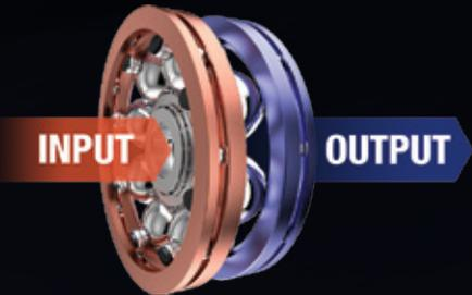
A set of spinning planets is fitted between an input ring, driven by the engine, and an output ring, which transfers power from the variator to the downstream drivetrain elements.
